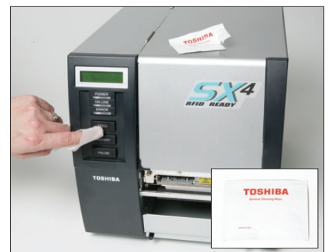
9. Close the printer and wipe the outside covers and panels with a dry Toshiba Cleaning Cloth. Remove external dirt with a Toshiba General Cleaning Wipe.
