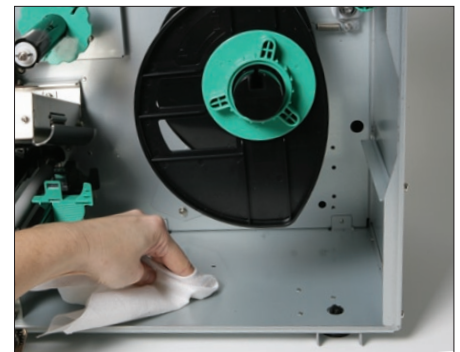
6. Clear any internal dust and debris with a dry Toshiba Cleaning Cloth.
