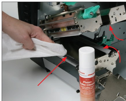
5. Spray some Platen Roller Cleaner on to a Toshiba Cleaning Cloth and gently wipe clean the platen, capstan roller and pinch roller.
