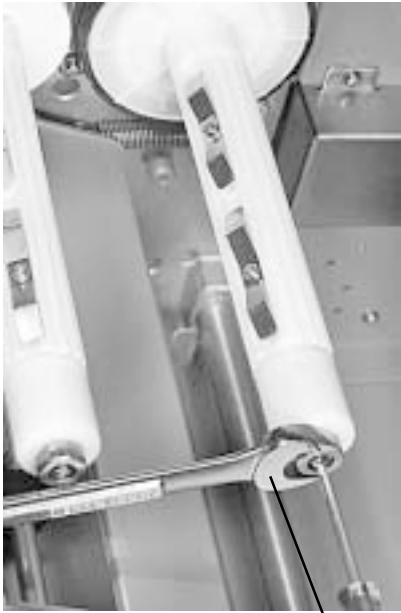
Fig. 6-41 USE 12mm OPEN END WRENCH AND PHILLIPS SCREW DRIVER TO REMOVE THE LOCKING SCREW AND ADJUSTMENT NUT
