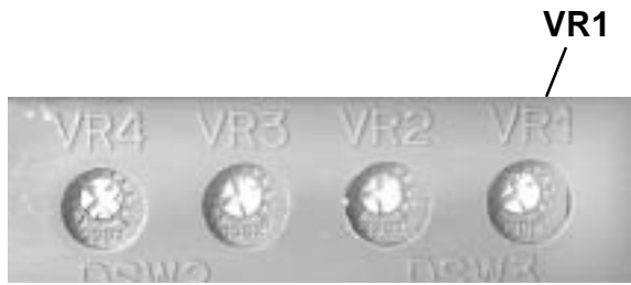
POTENTIOMETERS ARE LOCATED UNDERNEATH A FLIP - DOWN COVER ON THE FRONT PANEL
