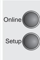
Press the **Setup** key. The printer changes to setup mode.
