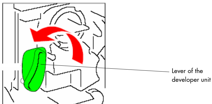
Fig. 7.1.2.b Detail: Unlocking the developer unit
