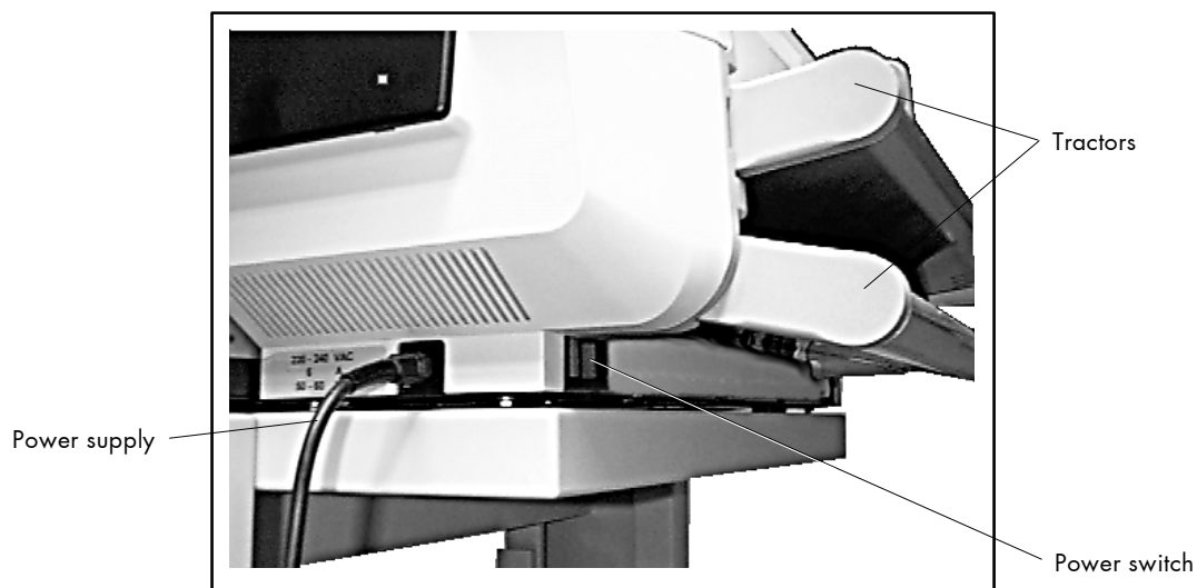
Fig. 5.2.a Turning on the printer (printer's rear view)
