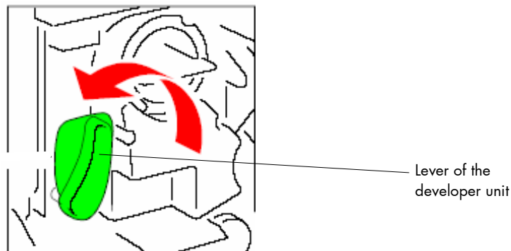
Fig. 2.4.2.b Detail: Unlocking the developer unit
