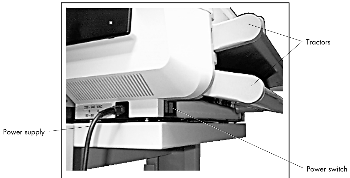
Fig. 2.2.b Printer's rear view: power supply
