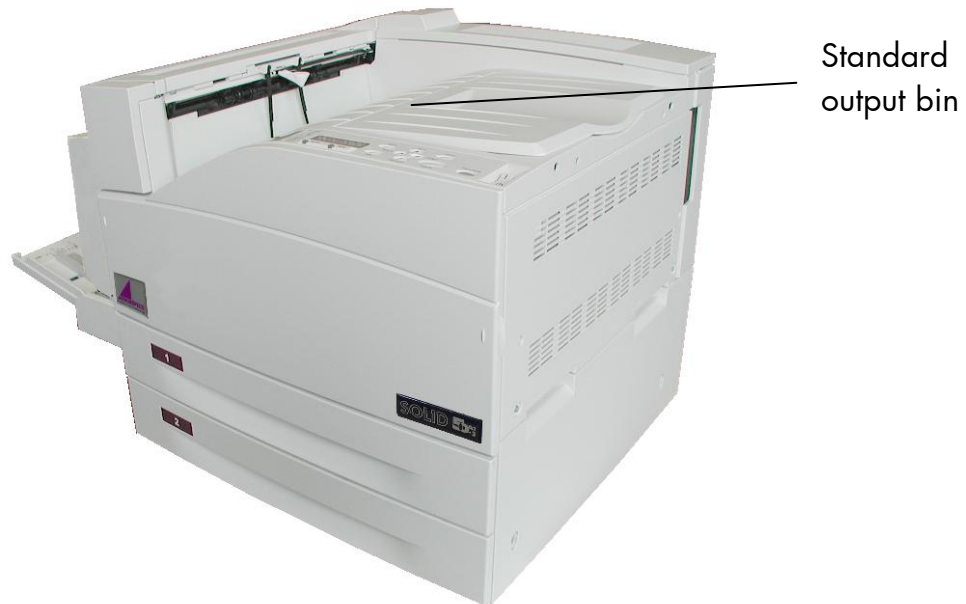
Fig. 3.1.3.a Standard output bin of the printer
