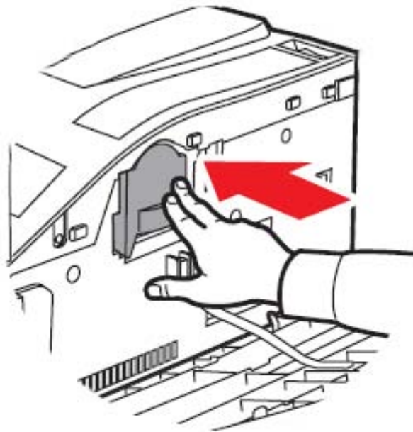
Fig. 2.3.l Inserting the new toner cartridge
