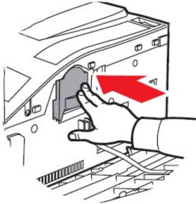
Fig. 3.2.g Inserting the new toner cartridge
