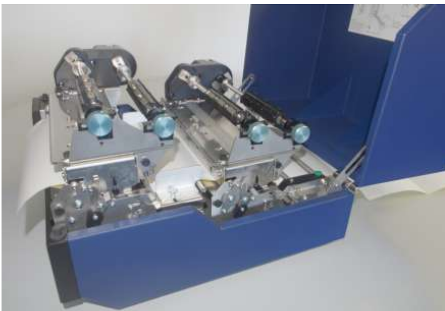
Fig. 5.1.1.m Both printhead assemblies are swivelled down and locked
