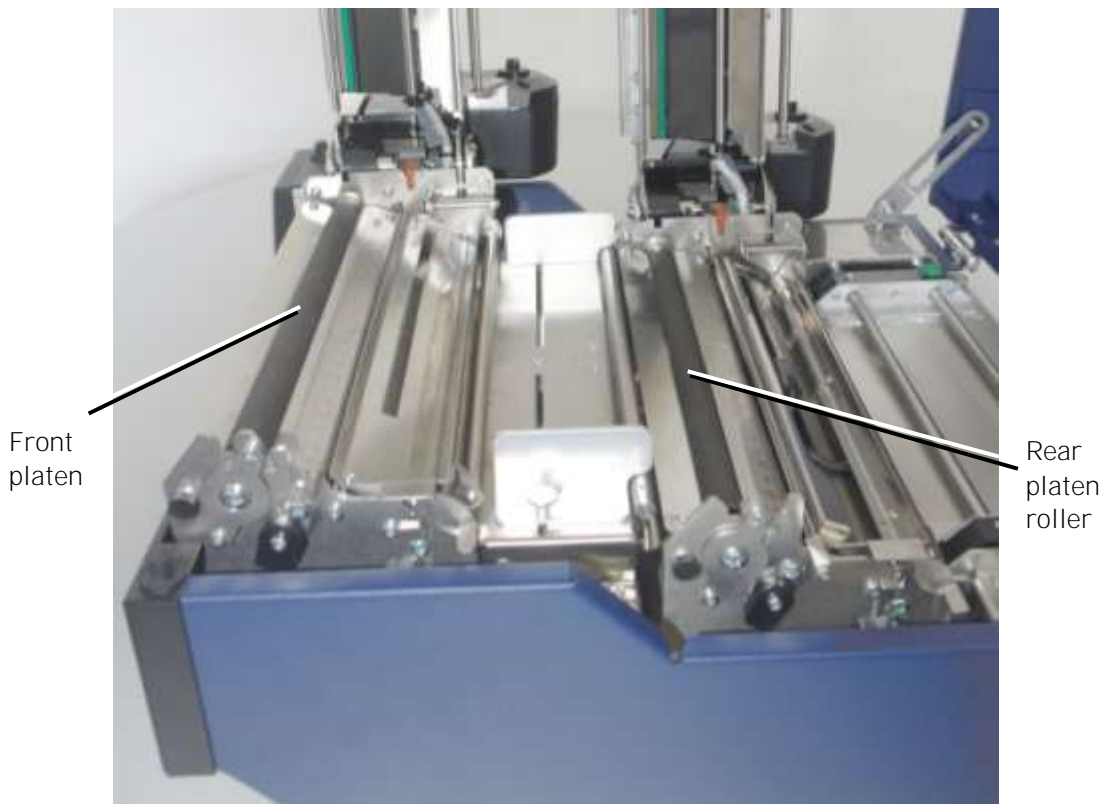
Fig. 8.1.3.c Position of the platen rollers
