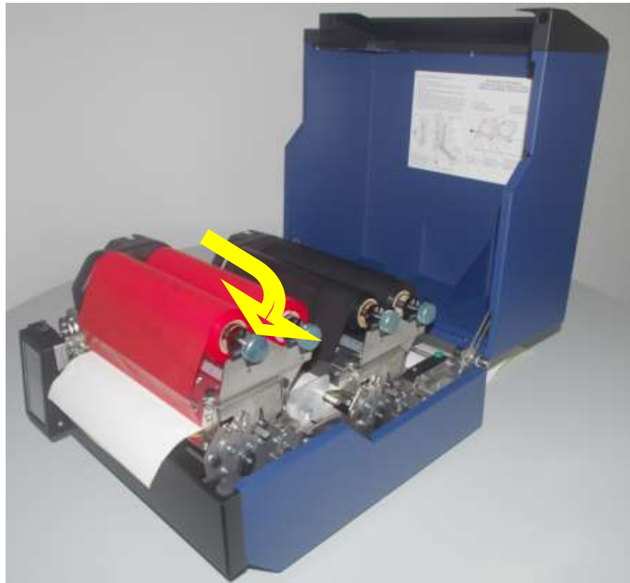
Fig. 5.2.2.k Printer with ribbons installed
